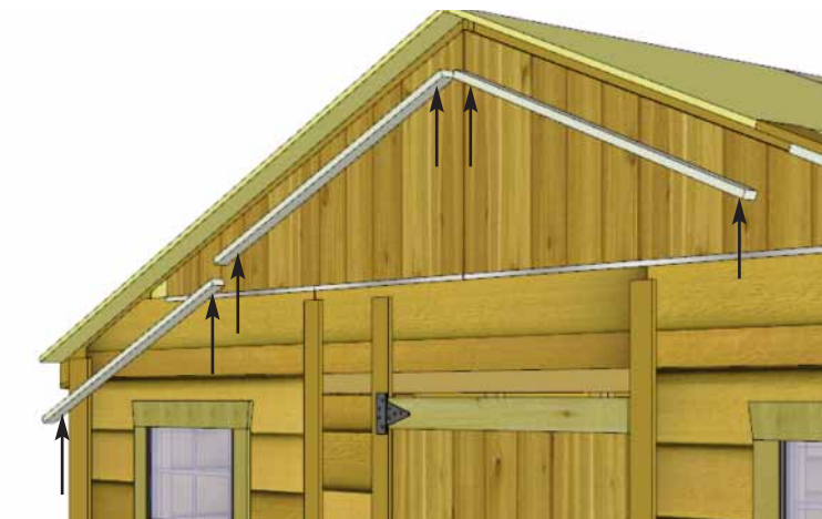
78. Attach Facia Cleat (3/4" x 1 1/2" x 36 1/2") centered on underside of Short Roof plywood, flush to edge. Attach Facia Cleats (3/4" x 1 1/2" x 40") to underside of Long Roof plywood, 1/2" from ends and flush to edge. Repeat this step on the rear side of shed. Fasten with 3 - 1 1/4" screws per piece.
