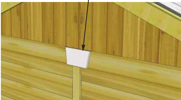
Horizontal Gable Detail Plate
