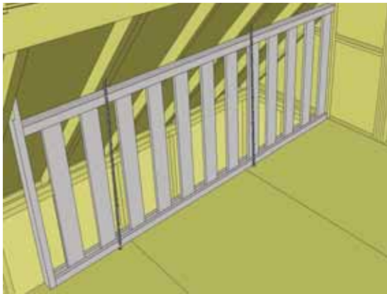
Completed Safety Railing
