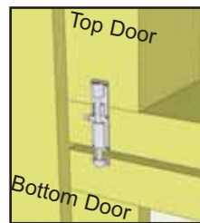
G. Attach Barrel Bolt to Top and Bottom Doors with 3/4" silver screws.
