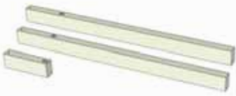
A - Canopy Lowering Cleat - 3 Pcs. - 1 1/2" x 2 1/2" x 33 5/8" x 2pcs - 1 1/2" x 2 1/2" x 8 1/2" x 1pc
