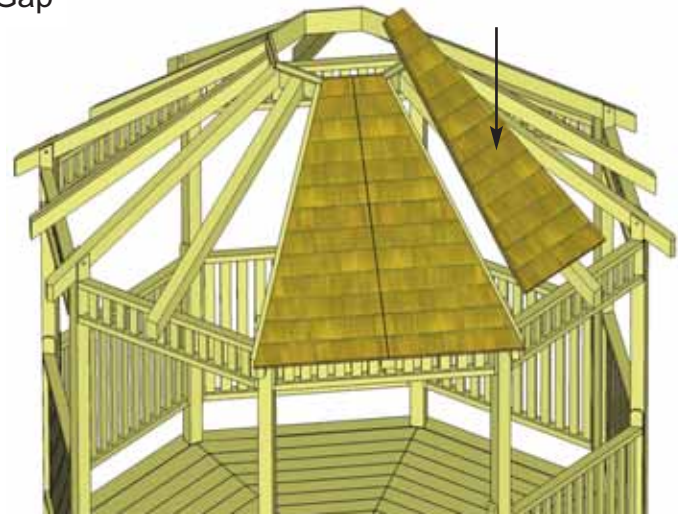
70. Lift and place 2nd Left Side Roof Panel in adjacent pie shape section.
