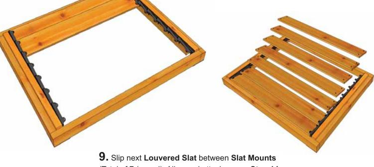
(Total of 7 / panel). Align and attach as per **Step 14.** Complete remaining Slats.
