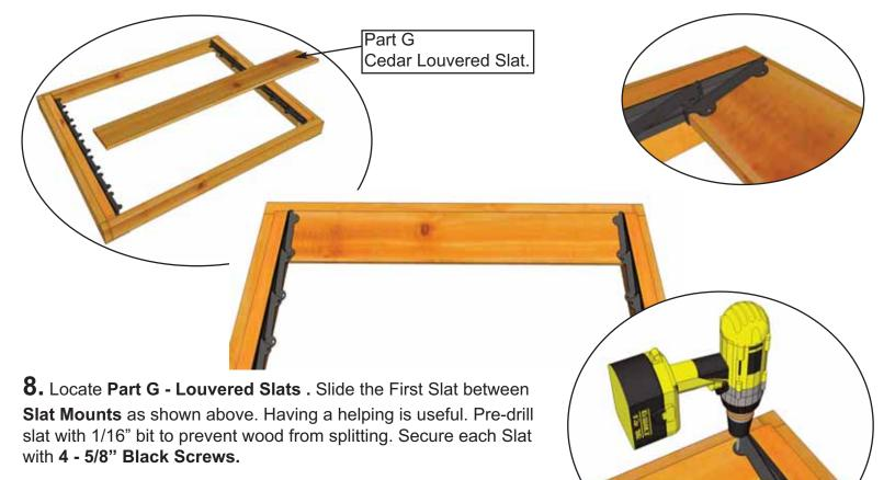
**Note -** Before securing Slats, observe how each is manufactured. Edges on faces can be slightly different. Sort and orientate all Slats so when creating your Louvered Panel all are orientated similarly.
